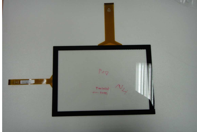
TP 產品背面照片 (Bottom view of touch panel)
